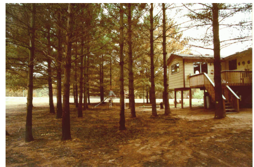
This home survived a wildfire because the trees were pruned & thinned and underbrush cleared.
