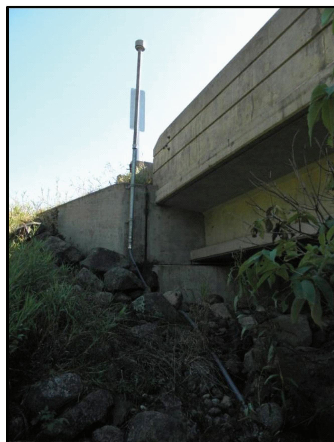
Figure 2. USGS stream gage installed on the St. Louis River.
