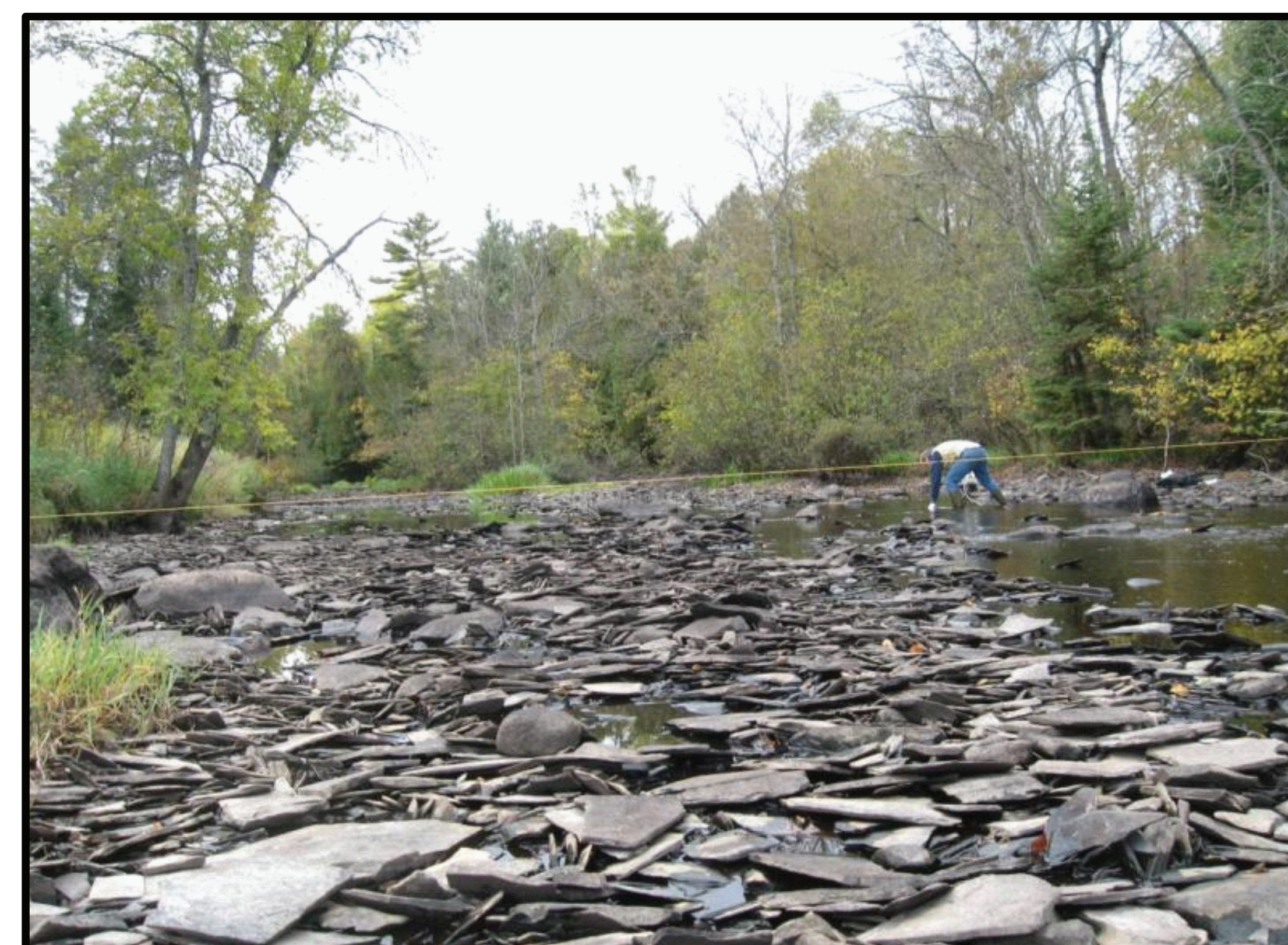
Figure 4. Streambed-sediment sampling in the St. Louis River. At this location, outside of the Duluth Complex, the river flows over graywacke and shale of the Virginia Formation.
